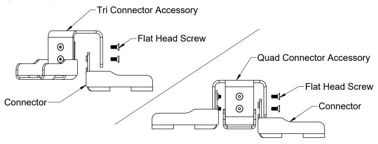
**Step 3:** Place the assembled Connector onto the ground. Then carefully dock the Stroll T-Base unit onto the assembled Tri or Quad Connector as shown. Please note for safe use the Stroll T-Base unit should always be docked in the Connector when in use.
