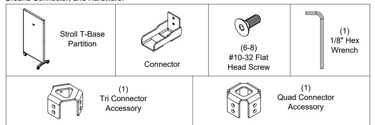
**Step 2:** Using two Flat Head Screws install one Connector onto the Connector Accessory as shown. Repeat this step until all Connectors are attached.
