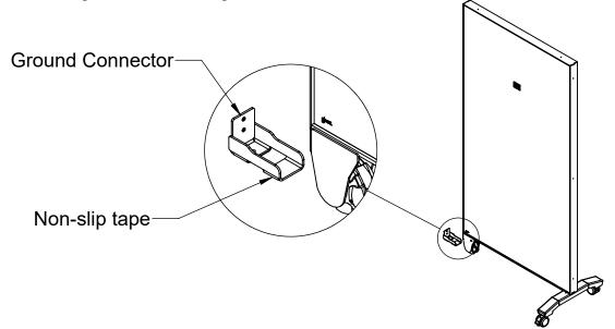
**Step 3:** Carefully roll the Stroll T-Base unit onto the Connector as shown. Please note for safe use the Stroll T-Base unit should always be docked in the Connector when in use.
