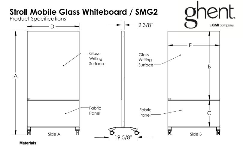
Board Surface: 1/8" thick, tempered low iron glass
