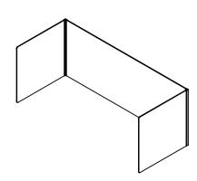
**Step 5:** Remove the tape backing from Feet and attach one to the bottom of the Side Panels as shown. Repeat for remaining panels. Clean and dry the tabletop before adhering the tape to the tabletop.
