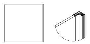
**Step 3:** Lay the Large Panel onto a clean flat surface. Press the Angle Connector onto the short side of the panel as shown.
