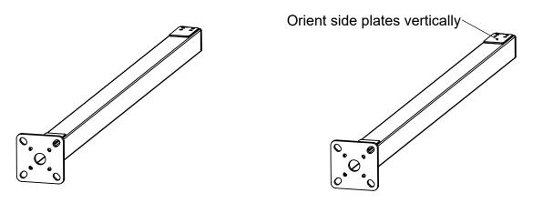
**Step 3:** Attach the Awning Arms onto the Side Posts as shown. Ensure that the Awning Mount holes and the Side Plates are oriented vertically.
