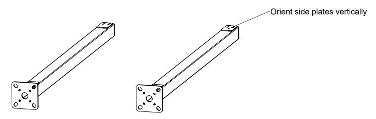
**Step 3:** Attach the Awning Arms onto the Side Posts as shown. Ensure that the Awning Mount holes and the Side Plates are oriented vertically.
