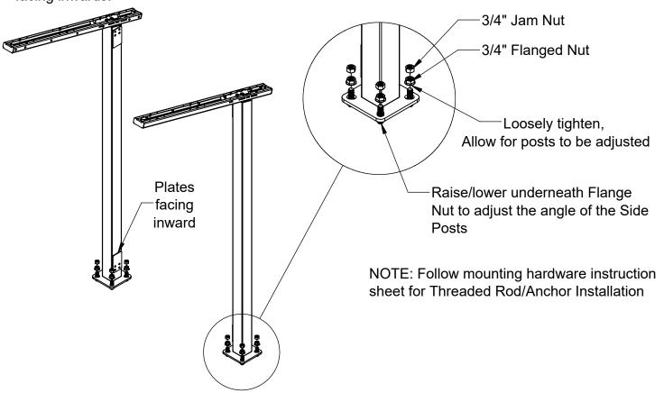
**Step 5:** Add the Crossbraces as shown below. Use the provided Tamper Resitant Hex bit and tool. After tightening, fully tighten 3/4" Nuts on Side Posts
