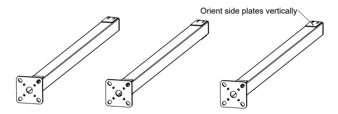
**Step 3:** Attach the Awning Arms onto the Side Posts as shown. Ensure that the Awning Mount holes and the Side Plates are oriented vertically.
