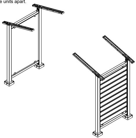
**Step 8:** Install 72" Awning Arms. Ensure the 72" Awning Arms are above 54" Awning Arms. Use Angled Alignment Mounts. If Top Awning Arms do not align, adjust the Side Awning Arms where they meet the Side Posts until aligned. If this is not sufficent, refer to Step 4 and adjust the underneath Flange Nuts until the arms are aligned.
