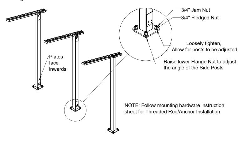
**Step 5:** Add the Crossbraces as shown below. Use the provided Tamper Resitant Hex bit and tool. After tightening, fully tighten 3/4" Nuts on Side Posts
