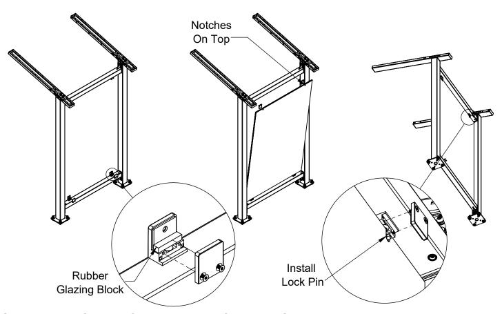
**Step 6B:** Install Slat Wall if applicable. Note: Crossbrace Screws may need to be adjusted when installing Slat Wall. Fully tighten these bolts when finished.
