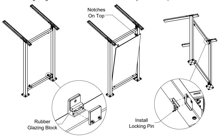
**Step 6B:** Install Slat Wall if applicable. Note: Crossbrace Screws may need to be adjusted when installing Slat Wall. Fully tighten these bolts when finished.
